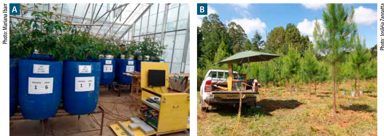
Figure 4.7. Cavity ring-down spectroscopy (CRDS) analyzer for monitoring greenhouse gas flows in soil planted with forest species in a greenhouse (A) and in the field (B), both at Embrapa Forestry.
